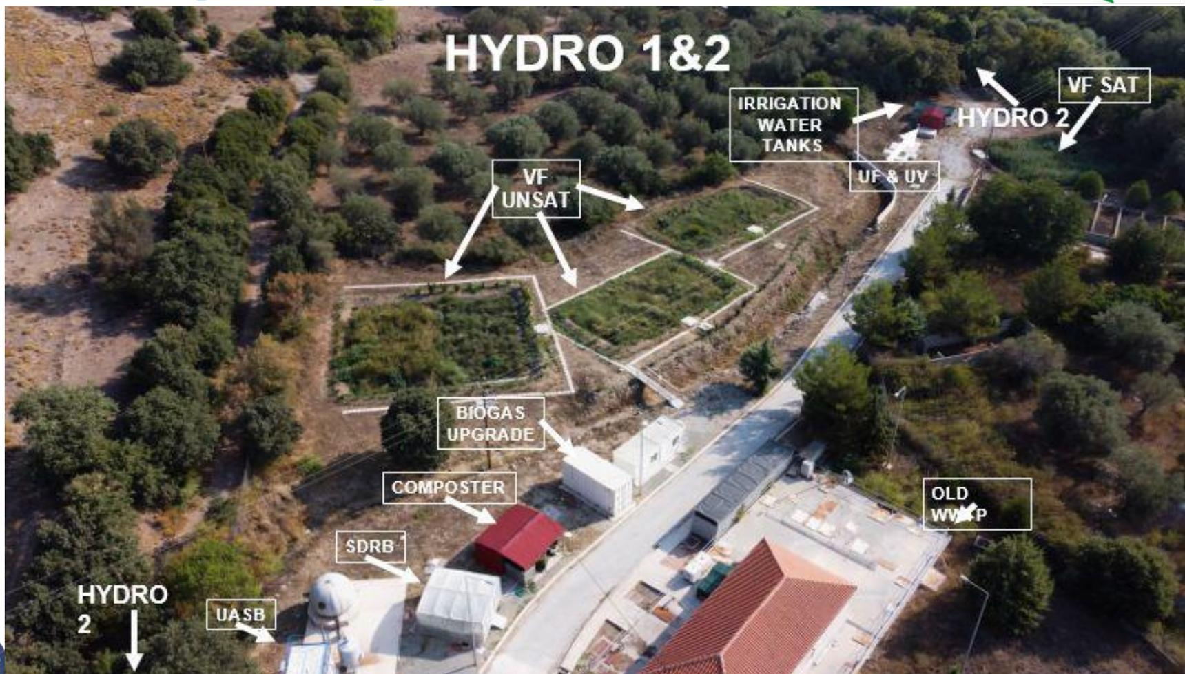
**Q: 10 – 100 m<sup>3</sup>/d; area UASB: 30 m<sup>2</sup>; area CW: 850 m<sup>2</sup> (virca 2 m<sup>2</sup>/PE)**
