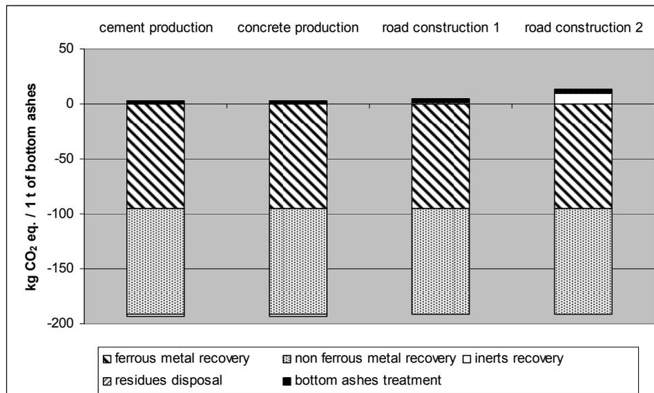
Figure 3: Contribution of each sub-process to the Global Warming Indicator (GWP<sub>100</sub>) for the treatment of 1 tonne of bottom ashes.
