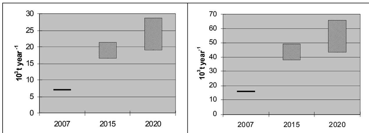
Figure 2. Aluminium recoverable from bottom ashes (left: conventional technologies; right: advanced technologies).
